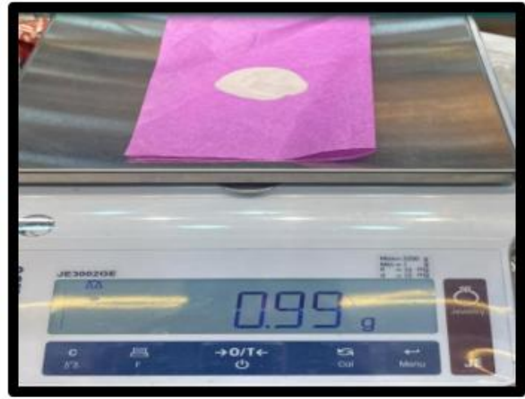
Fig. No. 10: Weighing the specimen soft liner
